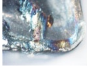
Built-up edge (Adhesive wear)
