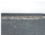
Thermal cracks (Thermal wear)
